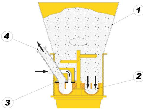
1. The dry material is fed through the hopper down into the pockets of the rotary feed wheel below.
