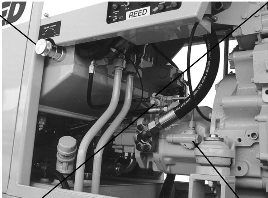
PRESSURE COMPENSATOR ADJUSTMENT (MAIN SYSTEM)
