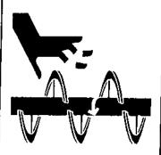
Keep hands out of hopper and valve assembly. See operation manual if access is required.
