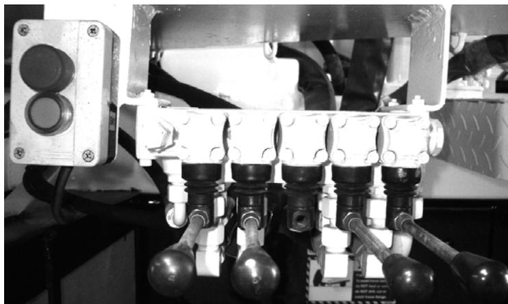
Movement direction of the outrigger and jacks is determined by upward or downward movement of the lever. Fully extend outriggers and use jack cylinders to stabilize machine within 3° of horizontal.
