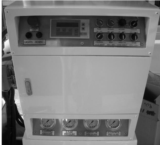
The control panel located on the deck features switches to control Emergency Shutdown, Forward Pumping, Reverse Pumping, Pumping Output, Engine RPM, Hydraulic Oil Cooling Fan, Local/Remote Control, Lights, S-Tube Shift, Drive Cylinder Extension, and Horn. A text display is also on the control panel to gauge engine RPM.
