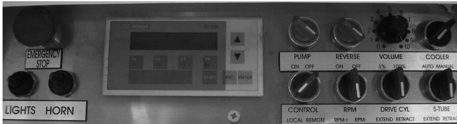
Concrete pumping operations are controlled utilizing the system control box. See description of each function below:
