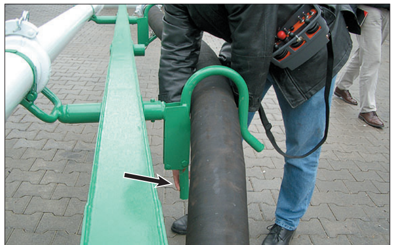
Fig. 7.17 Release the discharge hose
