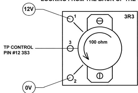
WIRE PROCEDURE FOR POTENTIOMETER USED ON C-SERIES CONTROL BOXES
