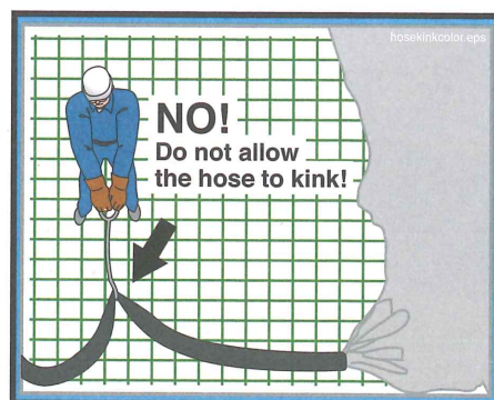
Figure 19 Kinking the hose creates a hazard
