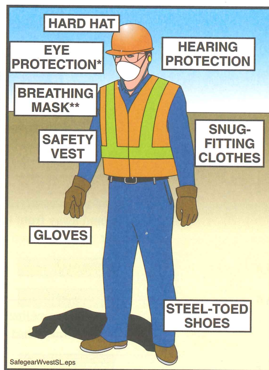
Figure 50 Wear Personal Protective Equipment (PPE)
