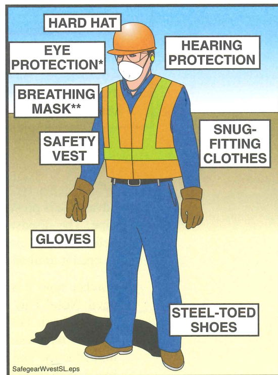
Figure 14 Wear Personal Protective Equipment (PPE)
