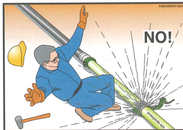
Figure 52 Never open a pressurized pipeline
