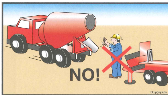
Figure 41 Never stand between the ready mix truck and the pump
