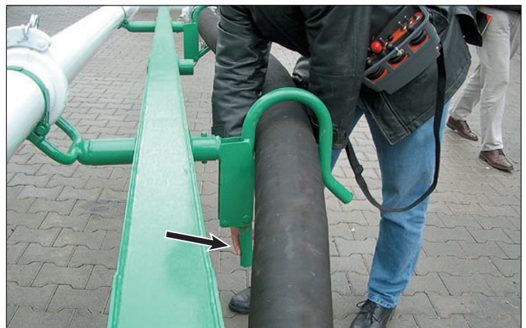
Fig. 7.17 Release the discharge hose
