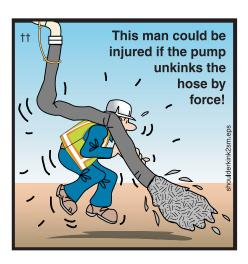
Figure 49 Kinking the hose creates a hazard
