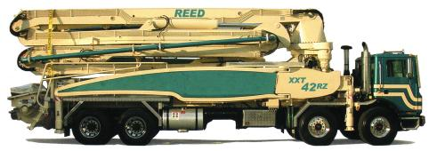
**Boom:** Versatile, compact, fully articulating 5-section RZ-fold boom represents the latest in boom technology. Radiused boom design to improve durability and eliminate stress focal points. Low unfolding height of 28′ (8.53 m).
