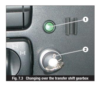
To drive the hydraulics a definite gear must be selected as shown in the information plate.
