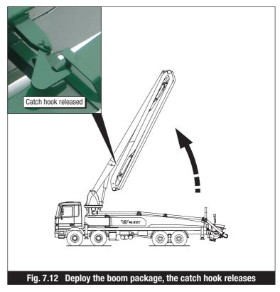
Press the boom rotation control lever (Item 9, Fig. 7.11) to rotate the boom package into the working position.
