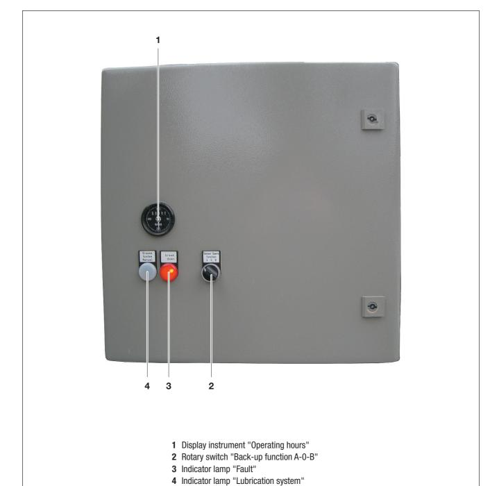
Fig. 5.7 Control cabinet control panel
