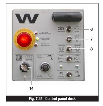
If the Emergency Stop button has been pressed, provided all Emergency Stop buttons has been released, the controls will be switched on again (reset).
