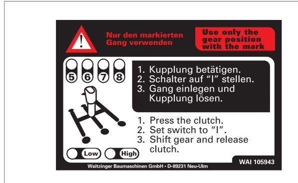
Fig. 2.38 Item 22 - WAI105943 - Disengage the clutch
