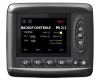
ALTERNATE CONTROL MODE - Selecting REMOTE when there is an error will allow normal remote controls. Pressing the OK Button toggles REMOTE and LOCAL.
