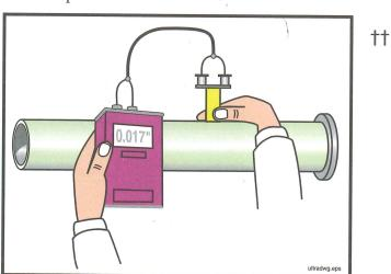
Figure 36 Check delivery system wall thickness with an ultrasonic thickness tester
