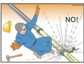
• Do not use compressed air to blow out concrete delivery hose, single pipe sections and short pipelines up to a length of 40 feet. Hoses will jump and
