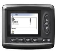
Selecting INFO provides the operator with 2 more options, See the list of Modules and status (Above) and See the system logs of operation and/or errors that have occurred during operation. (Below)
