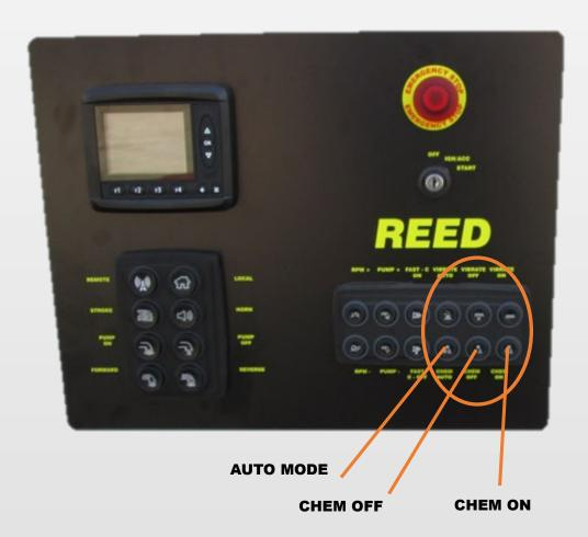
THESE CONTROLS ARE USED FOR (OPTION SYNCHRONISED CHEMICAL PUMP)
