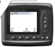
Main Menu Screen - After pressing the menu button a screen appears that provides the operator three options Adjust, Preferences, and Info
