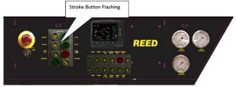
Alternate Control Mode - If at any time the pump detects a loss of communication to the 2X4 or 2X6 control button pads or with the MVEC relay box it will assume there has been a failure of one or more of
