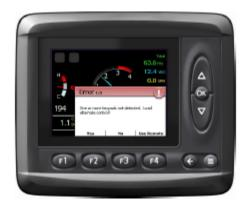
PROX OVERRIDE MODE - Select Override from the popup (above) Stroke button will be flashing to indication Override mode. (Below)
