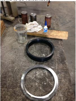
2. Clean surfaces, then apply Loctite in approx 1/4" bead where the two parts will touch
