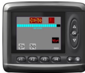
DEF TANK LEVEL
