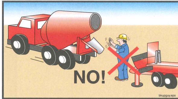
Figure 41 Never stand between the ready mix truck and the pump
