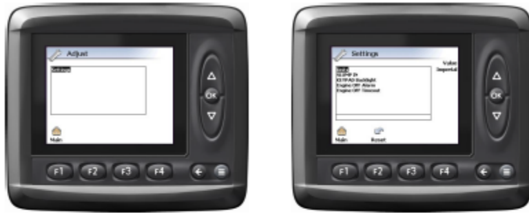
Selecting ADJUST provides the operator the ability to make setting to basic pump features (Above)
