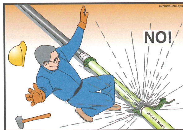
Figure 52 Never open a pressurized pipeline
