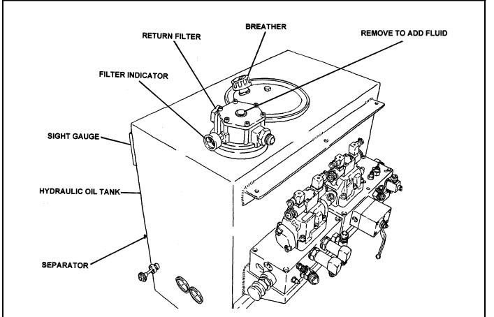
The purpose of installing hydraulic filters in the system is to provide a means of continuous hydraulic fluid filtration in an effort to prevent recirculation of abrasive solids which will cause rapid wear of component breakdown.
