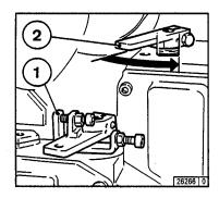
Move speed control lever 1 to low idle.
