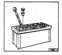
• Measure the specific gravity of individual cells with a commercial hydrometer.
