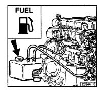
Use only commercial-grade diesel fuel. For fuel grade, see 4.2. If required use a preliminary fuel filter.
