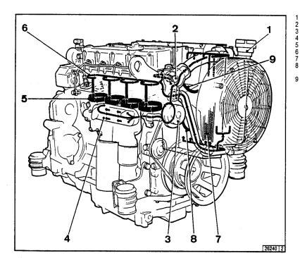
Thermostat housing Coolant pump Lube oil cooler
