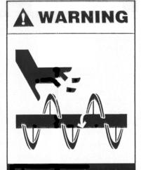
Keep hands out of hopper and valve assembly. See operation manual if access is required.
