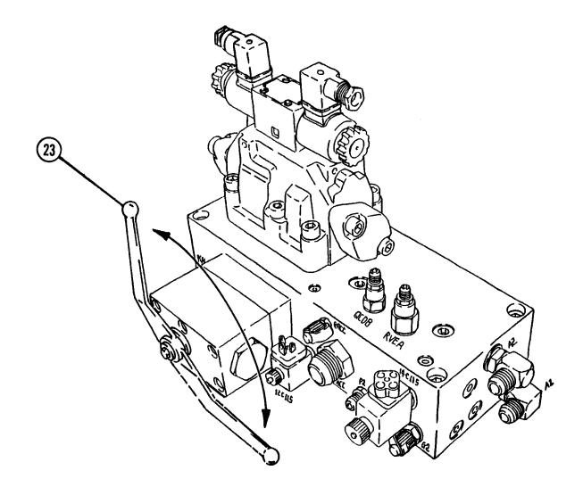
For an easier, slower shift, move the ball valve lever to the 3 o'clock position. This closes the ball valve and directs the fluid through the orifice. This position may be used when a slurry is being pumped or when the machine is being cleaned out.
