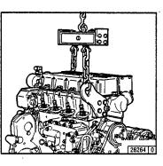
• Always use proper lifting tackle when transporting the engine.
