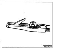
The V-belt tension gauge can be obtained under order number 8115 + 8120 from:
