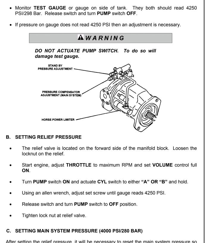
After setting the relief pressure, it will be necessary to reset the main system pressure so that it is lower than that of the relief pressure.
