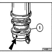
Fill oil cup 1 of the oil bath air cleaner (if fitted) with oil up to the arrow. For oil grade and viscosity, see 4.1.
