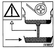
Place an oil tray beneath the engine
