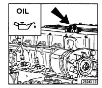
As a rule, engines are delivered empty of oil. Pour lube oil into the oil filler neck (arrow). For oil quantities, see 9.1. For oil grade and viscosity, see 4.1.
