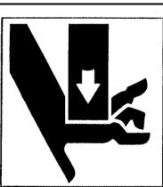
Keep hands out of waterbox. Stop engine/motor if access is required. Keep guards in place.
