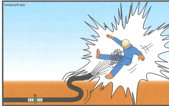
Figure 33 Never use air to blow out hoses or short pipelines
