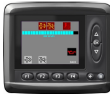
DEF TANK LEVEL
