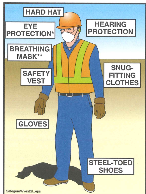
Figure 40 Wear the same personal protective equipment as the operator
