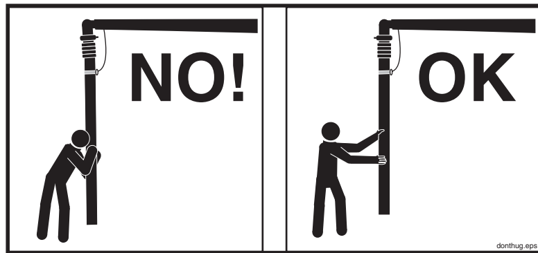
Figure 84 Do not hug the boom hose
