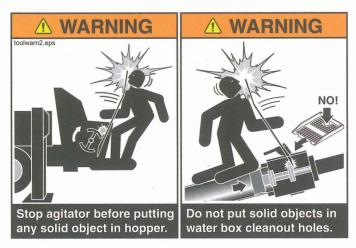
Figure 28 Don't put solid objects into working systems
