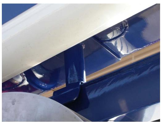
Trimmed Section Rest (In between C and D sections): New Overall Length 6 7/8" Plate for Section Rest: 3 3/4" x 6" x 3/8"
