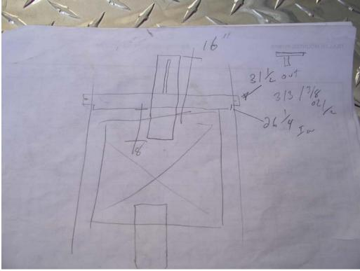
Rough Sketch for Boom Skid Plate (Protect Cooler from Settling Boom)
