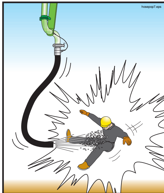
Figure 47 Remove everyone from the discharge area whenever air is in the line
