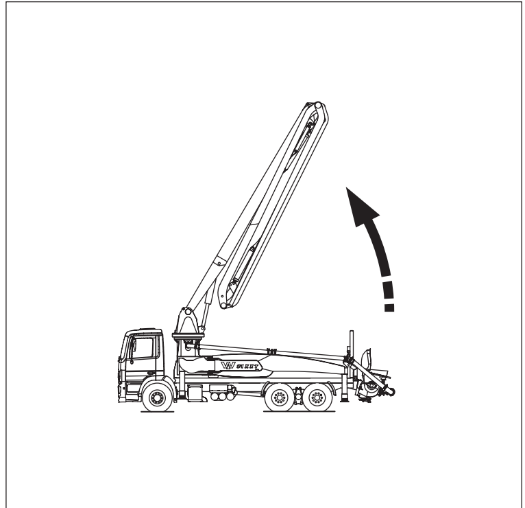
Fig. 7.12 Deploy the boom package, the catch hook releases
