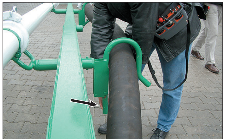
Fig. 7.17 Release the discharge hose
