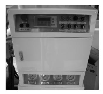
The control panel located on the deck features switches to control Emergency Shutdown, Forward Pumping, Reverse Pumping, Pumping Output, Engine RPM, Hydraulic Oil Cooling Fan, Local/Remote Control, Lights, S-Tube Shift, Drive Cylinder Extension, and Horn. A text display is also on on the conrol panel to gauge engine RPM.
